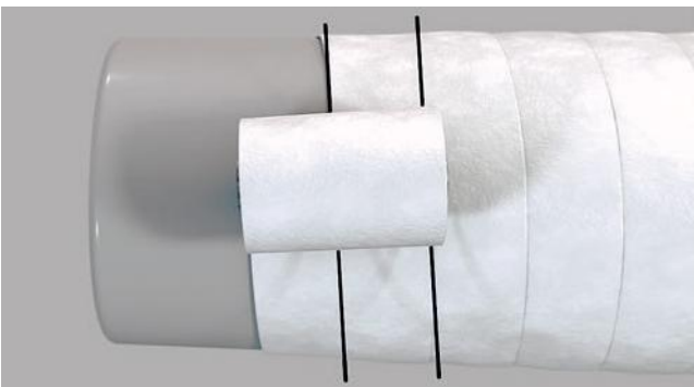
Fig 14.1-40 The half-overlapping technique.
