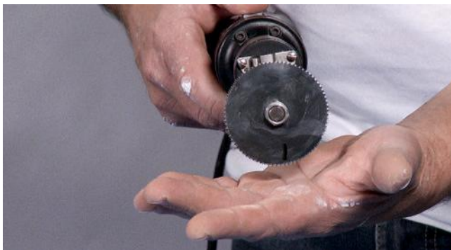
Fig 14.1-48 The saw blade oscillates and does not rotate, so the risk of skin injury is reduced.
